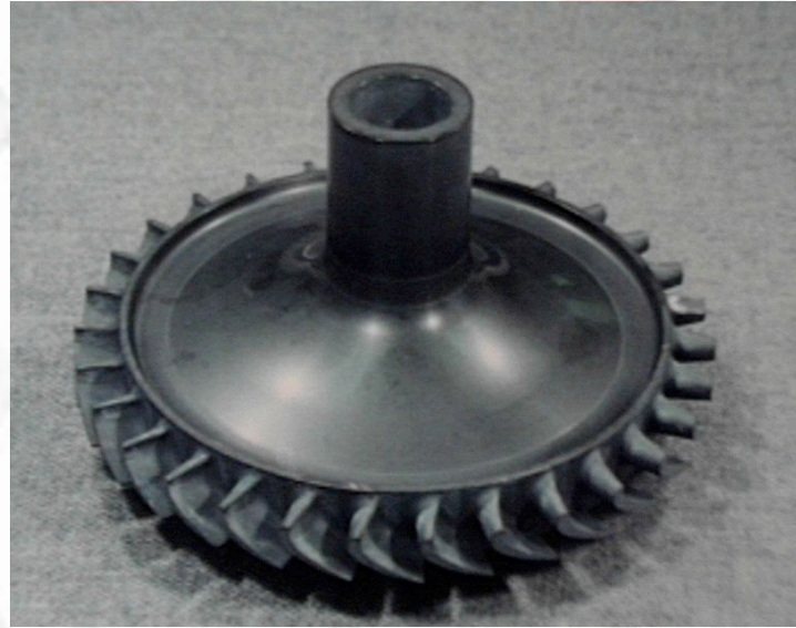
Figure 2. Silicon Nitride Turbocharger Rotor
